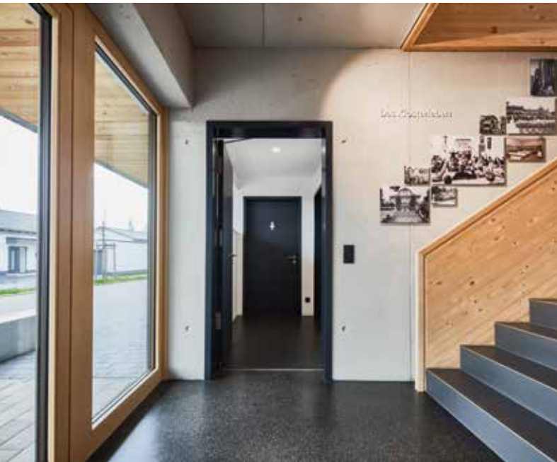
The door leaves in the sanitary areas are equipped with an ABS edge.
