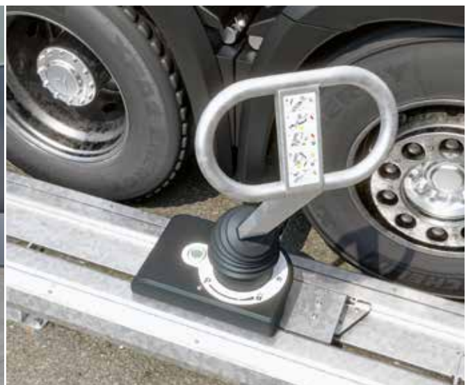
The loading site is only cleared once direct tyre contact is made.
