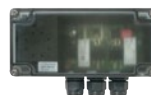
2-channel relay receiver HET-E2 24 BS 2 volt-free relay outputs for choosing the direction, one 2-pin input for volt-free Open and Close limit switch reporting (for querying the door position)
