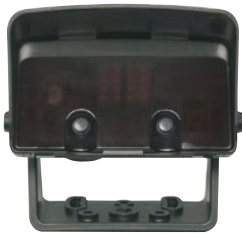
Radar movement detector MWD-C Fast and targeted automatic door opening, directional recognition, max. fitting height 7 m, fitting in deep freeze area possible to max. -22°C, IP 65
