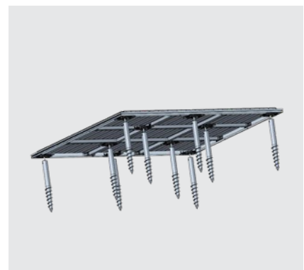
Juno screw foundation The screw foundation contains the ground screws. Support brackets, fixing material and the screw-in aid The bottom frame, the floor base construction and the floor (or optionally a 2 cm thick support made of timber, OSB board or resin-impregnated plywood plate provided on site) are also required.
